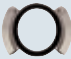
Figure 2: The lugs in this illustration are referred to as "ear lugs". "Ear lugs" are used for inlets and in suction operations.
